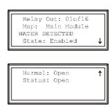
The Main Module supports up to 16 user-defined output relays. Output relays respond to internal alarms and events by changing state to notify outside devices.
